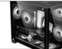
Top fans Mount 3 120mm fans or 2 140mm fans on the top, fix the fans with screws at the anchor points.
