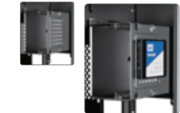
SSD 2.5" Find the slot for your SDD and install with the screws in the anchor points.
