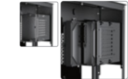
HDD 3.5" Find the slot for your HDD and install by sliding the drive into the tray then secure with the screws at the anchor points.
